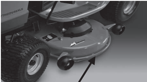
Armor Protected Stamped Deck Shell Example Below
