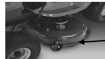
Stamped Deck Shell below, NOT reinforced
