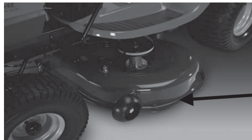
Stamped Deck Shell below, NOT reinforced
