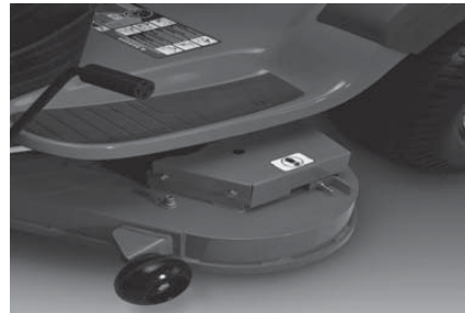
Fabricated Deck Shell Example Below
