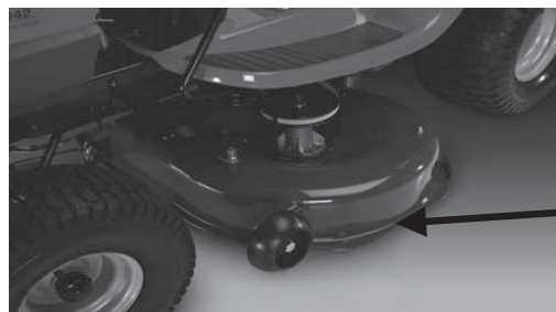
Stamped Deck Shell below, NOT reinforced
