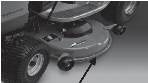
Armor Protected Stamped Deck Shell Example Below
