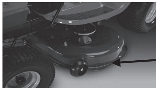
Stamped Deck Shell below, NOT reinforced
