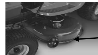
Stamped Deck Shell below, NOT reinforced
