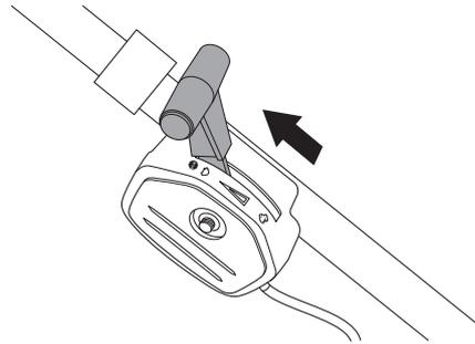
If the machine for any unexpected reason does not stop when the throttle control is moved to its stop position, disconnect the spark plug wire from the spark plug to stop the machine.
