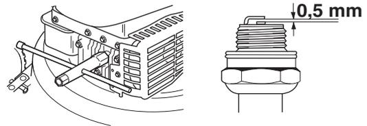
**CAUTION!** Always use the recommended spark plug type, refer to Technical Data. Use of the wrong spark plug can damage the piston/cylinder.
