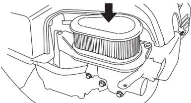
Clean the filter by knocking the filter against a flat surface. Never use solvents, for example petrol or kerosine, or compressed air to clean the filter.
