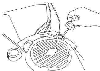
The oil filler cap must be completely screwed down to give a correct indication of the oil level.
