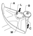
Screw on the trimmer head/plastic blades (H) in the opposite direction to the direction of rotation.
