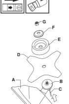
Hook the blade guard/combination guard (A) onto the fitting on the shaft and secure with the bolt.
