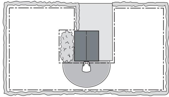
Do not put the charging station in confined spaces in the working area. There must be a straight boundary wire, at least 5 ft (1.5 m) long, to the right and left of the charging station. The wire must be laid straight out from the rear end of the charging station. Any other locations can mean that the robotic lawnmower enters the charging station sideways and will have difficulty docking.
