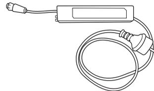
The low voltage cable for the transformer is 33 ft (10 m) long, and may not be shortened or extended.
