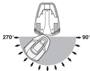
Two sensors, one on the front and one on the back of the robotic lawnmower, will sense when the robotic lawnmower is approaching the boundary wire. The robotic lawnmower travels up to 11" (28 cm) beyond the wire before it turns around.
