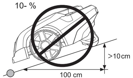
However, the boundary wire can be laid across a slope steeper than 10% if there is an obstacle that the robotic lawnmower is allowed to collide with, for example, a fence or a dense hedge.
