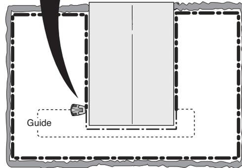
b) Put A1 and Guide back in their original positions. Then switch A2 and Guide.
