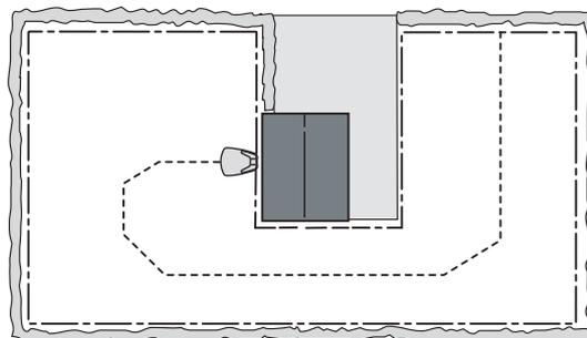
When the battery is fully charged, the robotic lawnmower leaves the charging station in a randomly selected direction within the 90°-270° exit sector.
