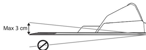
The charging station must not be positioned in a way that can bend its base plate.
