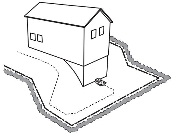
Avoid laying the wire at sharp angles. This can make it difficult for the robotic lawnmower to follow the guide wire.
