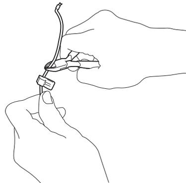
4. Press the connector onto the metal pins, marked with an A, on the charging station.
