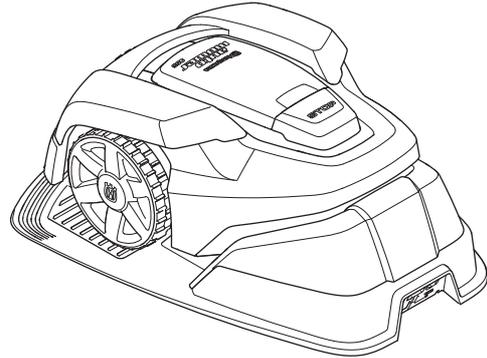
2. Park the robotic lawnmower in the charging station. Open the cover and push the robotic lawnmower in as far as possible to ensure proper contact between the robotic lawnmower and the charging station.
