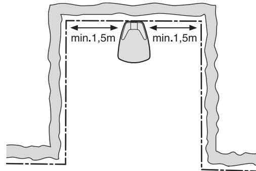
Do not put the charging station in a corner in the working area.
