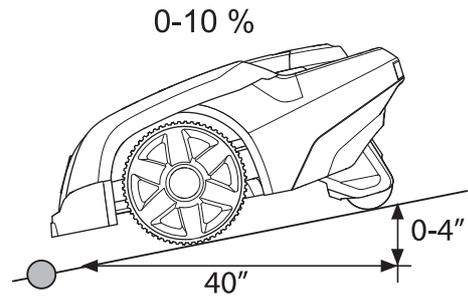
The boundary wire should not be laid across a slope that is steeper than 10%. There is a risk that the robotic lawnmower will find it difficult to turn there. The robotic lawnmower will then stop and the *Outside working area* fault message is displayed. The risk is at its greatest in damp weather conditions, as the wheels can slip on the wet grass
