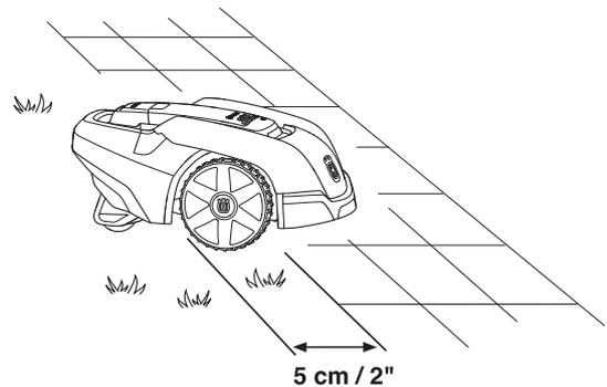
When the working area is divided by a paving stone path which is level with the lawn, it is possible to allow the robotic lawnmower to run over the path. It can be an advantage to lay the boundary wire under the paving stones. The boundary wire can also be laid in the joint between the paving stones.
