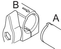
Push the attachment into the coupling until the attachment snaps into place.
