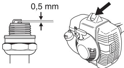
**CAUTION!** Always use the recommended spark plug type! Use of the wrong spark plug can damage the piston/cylinder.
