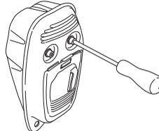
If the muffler on your machine is fitted with a spark arrestor screen this must be cleaned regularly. A blocked
