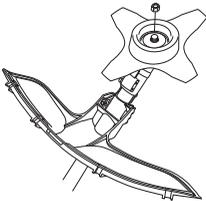
When fitting, tighten the nut in the opposite direction to the direction of rotation of the cutting attachment. To remove it, undo the nut in the same direction as the cutting
