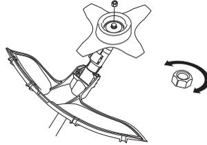
The nylon lining inside the locking nut must not be so worn that you can turn it by hand. The lining should offer a resistance of at least 1.5 Nm. The nut should be replaced after it has been put on approx. 10 times.
