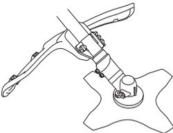
Check that the guard is undamaged and not cracked. Replace the guard if it has been exposed to impact or is cracked.
