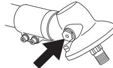
The grease in the bevel gear does not normally need to be changed except if repairs are carried out.
