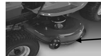
Stamped Deck Shell below, NOT reinforced
