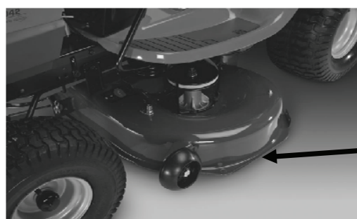
Stamped Deck Shell below, NOT reinforced
