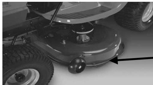
Stamped Deck Shell below, NOT reinforced
