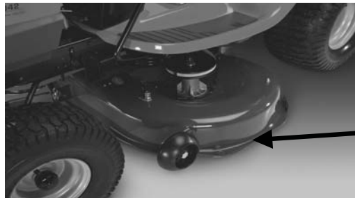
Stamped Deck Shell below, NOT reinforced
