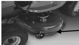
Stamped Deck Shell below, NOT reinforced
