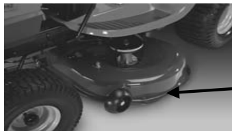
Stamped Deck Shell below, NOT reinforced
