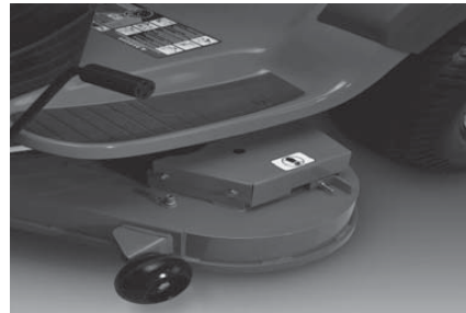
Fabricated Deck Shell Example Below
