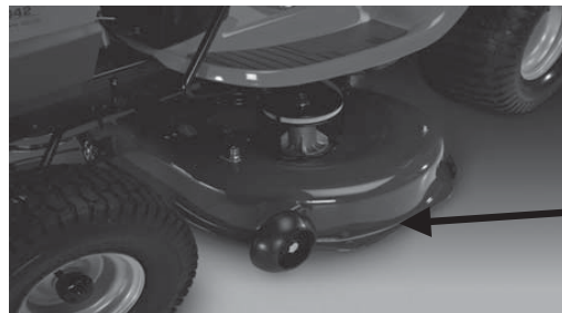
Stamped Deck Shell below, NOT reinforced
