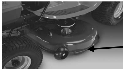
Stamped Deck Shell below, NOT reinforced
