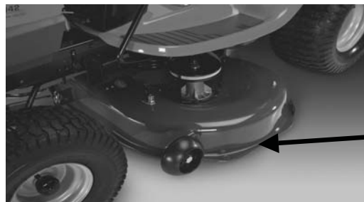
Stamped Deck Shell below, NOT reinforced
