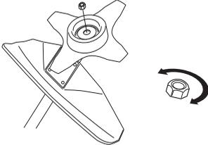
When loosening and tightening the saw blade nut, there is a risk of injury from the teeth of the saw blade. You should therefore always ensure that your hand is shielded by the blade guard when doing this. Always use a socket spanner with a shaft that is long enough to allow this. The arrow in the diagram shows the area where you should operate the socket spanner when loosening or tightening the nut.
