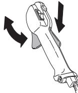
See instructions under the heading Start. Start the machine and apply full throttle. Release the throttle and check that the cutting attachment stops and remains at a standstill. If the cutting attachment rotates with the throttle in the idle position then the carburettor idle setting must
