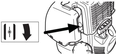
**Primer bulb:** Press the air purge repeatedly until fuel begins to fill the bulb. The bulb need not be completely filled.
