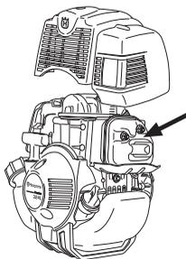
The muffler on your machine is equipped with a spark arrestor screen, this should be cleaned regularly. A blocked screen will cause the engine to overheat and may lead to serious damage.
