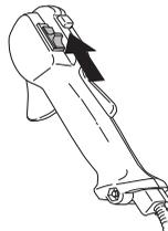
**Choke:** Set the choke control in the choke position.
