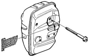
On mufflers without a catalytic converter the screen should be cleaned weekly, or replaced if necessary. On mufflers fitted with a catalytic converter the screen should be checked, and if necessary cleaned, monthly. **If the screen is damaged it should be replaced.**
