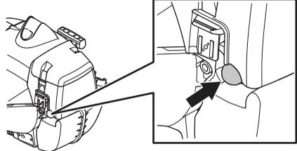
**Choke:** Set the choke control in the choke position.
