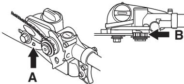
Tension the chain by turning the chain tensioning screw clockwise. Use a combination spanner or turn by hand. The chain should be tensioned until it fits snugly on the underside of the bar.
