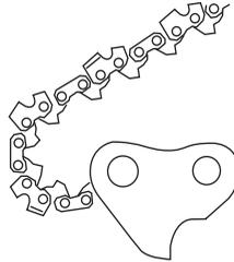
Level of kickback reduction. The only thing that describes the level of kickback reduction offered by a saw chain is its model number.
