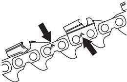
We recommend you compare the existing chain with a new chain to decide how badly the existing chain is worn. When the length of the cutting teeth has worn down to only 5/32 inch (4 mm) the chain must be replaced.
