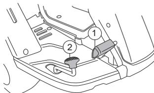
**Rider 112C5** has the brake pedal and lock button on the right hand side. Release the parking brake by first pressing down the parking brake pedal and then releasing it.
