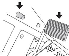
**For Rider 112C5** Disengage the engine and select the required gear.
