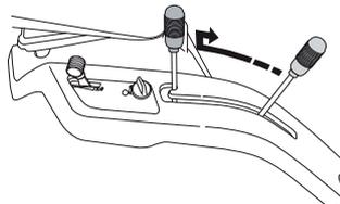
Pull back the throttle and let the motor idle for at least 30 sec.
