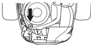
The dipstick should be **completely screwed down**
