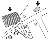
Carefully press down one of the pedals until the required speed is obtained. Pedal (1) is used to drive forwards, and pedal (2) to drive backwards.
