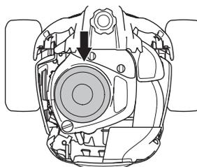
A blocked cooling intake will interfere with the cooling of the engine, which can damage the engine.
