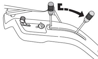
The lever can also be used to temporarily regulate the cutting height, e.g. for a small mound in the lawn.
