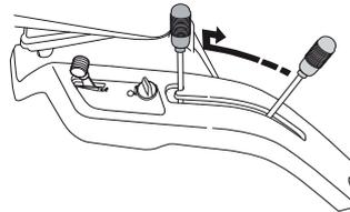
If the lever is moved forwards, the cutting deck will be lowered and the blades will automatically start to rotate (mowing position).
