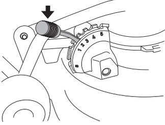
Lift up the cutting unit before adjusting the height.
