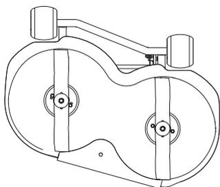
The blades should be balanced after sharpening.
