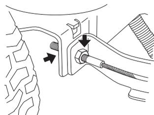
Hold the cable, for example using an adjustable wrench, so that it does not twist.
