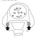
IMPORTANT! Never run the engine without the air filter fitted. The filters must not be oiled. They must be fitted dry.
