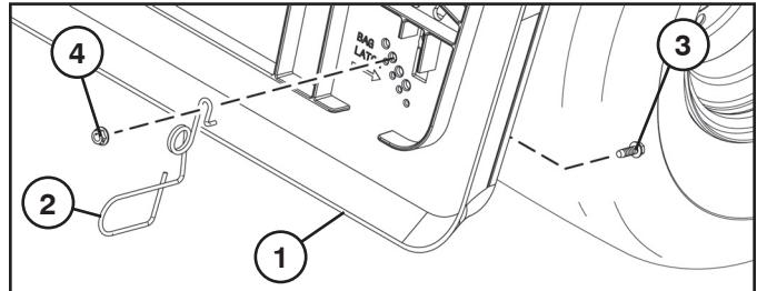
**NOTE:** The bottom of the bagger assembly should contact the loop end so that it is held securely when closed.
