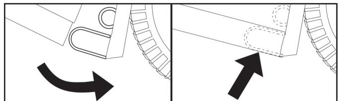
**NOTE:** If the bagger assembly height is adjusted, it may be necessary to adjust the bagger spring latch. To adjust, remove the nut (4) and move the bagger spring latch to the appropriate hole in the backplate (1), ensuring the bagger assembly will be securely closed. Retighten nut securely.
