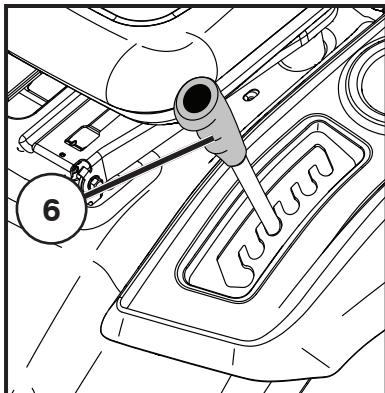
**GB 6. Quick lifting/lowering of the cutting unit**
