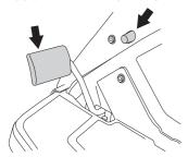
4 Check that the lever for setting the cutting height is in the S position.
