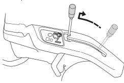
When the Rider is at a standstill, press down the parking brake and push in the locking button.
