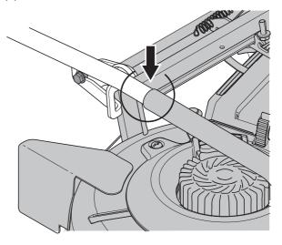
3 Press in the lock, grasp the pipes and slide in the cutting deck.
