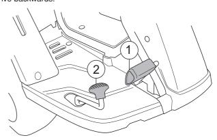
Pressing down both pedals stops the machine. Release both pedals and then press down the required pedal.
