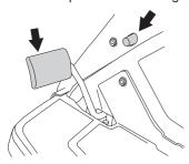
3 Turn off the machine by turning the ignition key to the "0" position.
