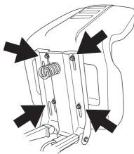
• Tighten the bolts after adjusting.
