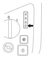
If the machine stops and has to be pushed to the charging station, the freewheel fuse in the rear carriage must be removed. Do not forget to put the fuse back in place before charging the battery.
