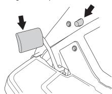
The parking brake lock disengages automatically when the brake pedal is pressed.
