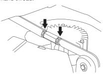
3 Screw out (extend) the strut to lower the rear edge of the cover.
