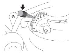
CAUTION! Lift up the cutting unit before adjusting the height.
