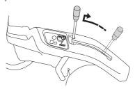
If the lever is pulled backwards the unit is raised and the blades automatically stop rotating (transport position).
