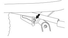
2 Fit the cutting deck's pipe together with the deck frame's pipe.
