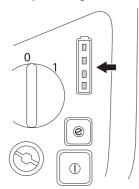
When all LEDs are lit the battery is fully charged.
