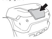
4 Connect the charger to the battery socket. The plug and socket fit only one way. Press in the plug and lock it in place.
