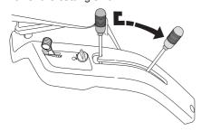
6 Loosen the snap lock for the covers on the cutting deck and loosen the cables. There are 2 for each motor.
