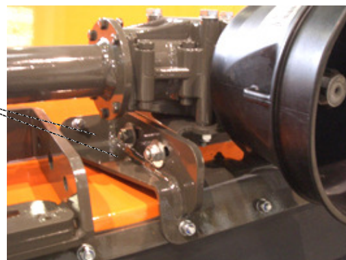
Illustration 22 Drive belt tensioning devices
