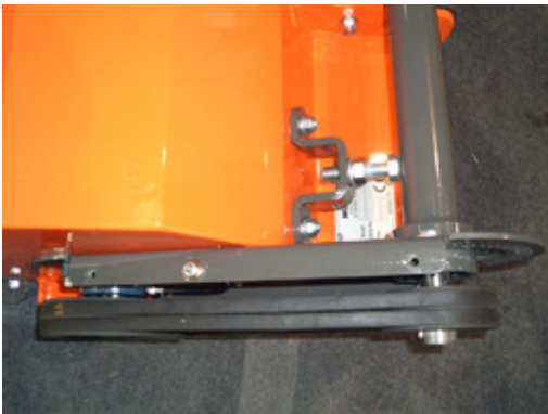
Illustration 26: pulley discs running in parallel
