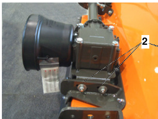
Illustration 24 Drive belt tensioning devices
