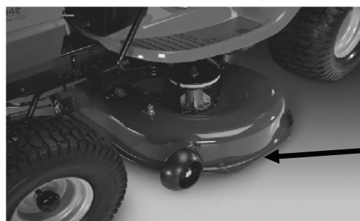
Stamped Deck Shell below, NOT reinforced
