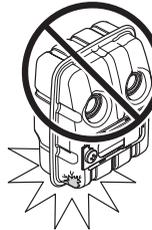
Regularly check that the muffler is securely attached to the machine.
