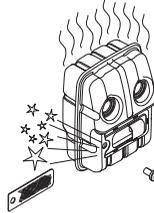
On mufflers without a catalytic converter the mesh should be cleaned weekly, or replaced if necessary. On mufflers fitted with a catalytic converter the mesh should be checked, and if necessary cleaned, monthly. **If the mesh is damaged it should be replaced.**
