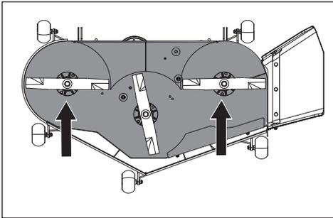
2. Measure from the floor surface up to the bottom of the blade tip on the discharge side of the mower deck. Record this measurement. Move to the opposite side; check that measurement is the same. If adjustment is required, loosen the locknut and adjust bolt up until both side-to-side measurements are equal. Retain measurement.
