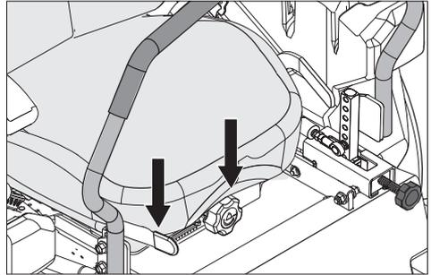
The seat can be adjusted lengthways with the lever located at the right side of the seat (as seen by the driver in the seat). When making adjustments the lever is moved upward.
