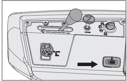
The service meter displays the total operating time with the blade activated.
