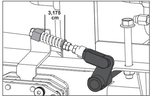
5. If adjustments are needed, loosen B jam nut and turn A jam nut until the correct distance is achieved. Retighten B jam nuts against A jam nuts.
