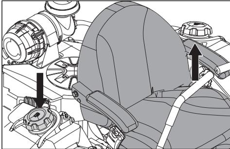
Read the safety instructions before refueling. The capacity for each tank is 20,8 liters.
