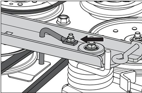
6. Remove the belt from around the electric clutch on the engine shaft.
