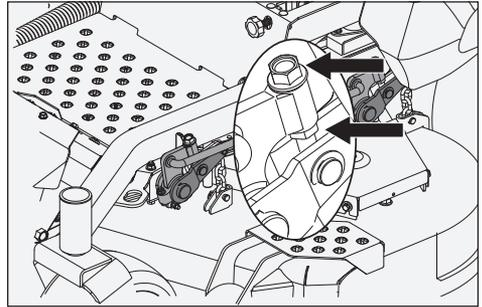
4. Confirm measurements once again. The blade tip height must be equal side-to-side. In the rear, blade tips must be 3,175 mm to 9,525 mm higher than the front measurement. In the front, blade tips must be equal from side-to-side.
