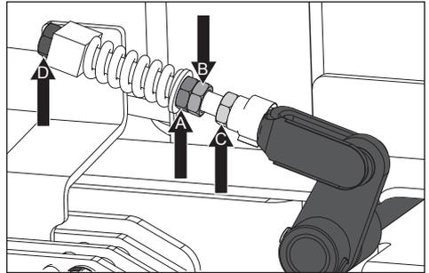
6. Engage the park brake. Measure the distance between the D brake bolt and the brake swivel. The distance must be 3,175 mm -6,35 mm.
