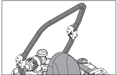
Operate the unit with the roll bar in the raised and locked position and use the seat belt. There is no rollover protection when the roll bar is down. If it is necessary to lower roll bar, do not wear the seat belt. Raise the roll bar as soon as clearance permits.
