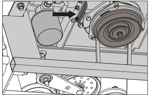
4. With a 1/2" breaker bar and using the square opening in the idler arm, shift the arm to create slack in the belt.
