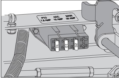
Fuses are located on the right hand side of the machine and are accessed by tilting the seat forward. Fuses are flat pin fuses type as used in automobiles. The 20 A is the primary fuse. The 7.5 A is for the mower deck coupling. The 10 A is for accessories.
