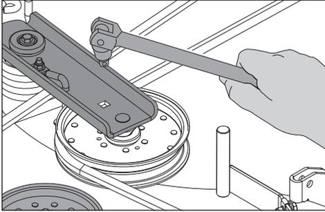
4. Carefully lift the belt over the top of the cutter housing pulleys.
