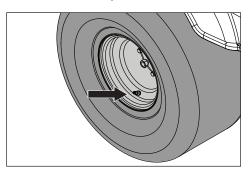
**IMPORTANT INFORMATION** DO NOT add a tire liner or foam fill material to the tires. Excessive loads created by foam filled tires will cause premature failures.
