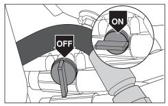
The fuel shut off valve is located at the left rear of the seat. The valve is off when the handle tab is turned perpendicular to the fuel line.
