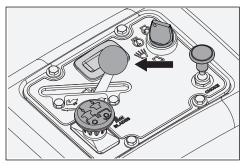
The throttle control regulates the engine speed and the rate of rotation of the blades, assuming the blade switch is pulled out.
