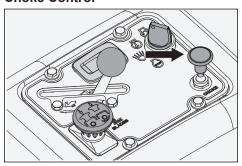
The choke control is used for cold starts to provide the engine with a richer fuel mixture. For cold starts, pull the control up.
