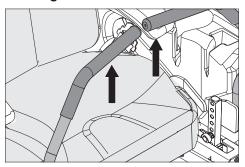
The machine's speed and direction are continuously variable using the two steering controls. The steering controls can be moved forward or backward about a neutral position. There is a neutral position, which is locked if the steering controls are moved out.
