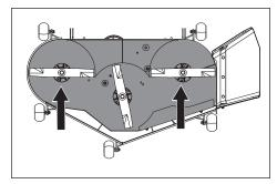
Measure from the floor surface up to the bottom of the blade tip on the discharge side of the mower deck. Record this measurement. Move to the opposite side; check that measurement is the same. If adjustment is required, loosen the locknut and adjust bolt up until both side-to-side measurements are equal. Retain measurement.
