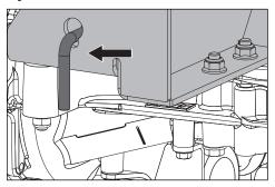
Transaxle bypass linkages must be engaged when pushing or pulling the mower. The release levers are located on each side of the rear of the unit below the rear engine plate. See *Manual Transport* in the *Operation* section.
