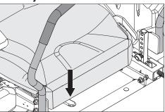
The seat can be adjusted lengthways. The lever under the front edge of the seat is moved to the left (as seen by the driver in the seat), to adjust the seat backward or forward.
