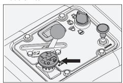
To engage the mower deck, pull the knob out; mower blades are disengaged when the knob is pressed down.
