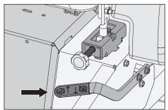
The park brake is found on the left of the machine. Pull the lever backward to operate the brake and push forward to release it.
