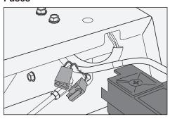
Fuses are located on the left hand side of the machine and are accessed by tilting the seat forward. Fuses are flat pin fuses type as used in automobiles. The 20 A is the primary fuse. The 7.5 A is for the mower deck coupling.
