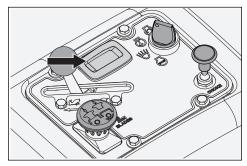
The service meter displays the total number of hours the engine has run and indicates when the engine and mower need servicing.
