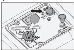
The ignition switch is placed on the control panel and is used to start and stop the engine. On models equipped with headlights, turn the key clockwise to ACCESSORY for headlight use.
