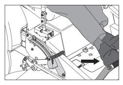
Activate the park brake, pulling the lever upwards.
