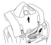
· Unscrew the plug on the grease nipple.
