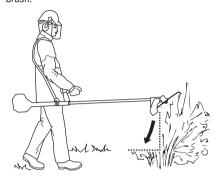
• The shredder blade must not be used on vegetation with a stem diameter larger than 2 cm.
