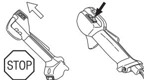
Start the engine and make sure the engine stops when you move the stop switch to the stop setting.
