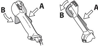
Make sure the throttle control is locked at the idle setting when the throttle lockout is released.
