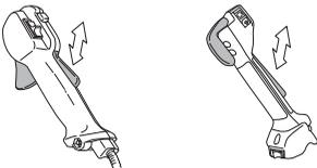
Check that the throttle trigger and throttle lockout move freely and that the return springs work properly.
