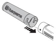
Push the tubes together and turn so that they lock together.
