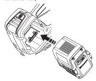
Press on the lower part of the battery and push it in as far as it will go into the battery compartment. The battery will lock itself into place when you hear a click. Make sure the latches snap in place properly.
