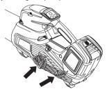
Check that the air intake is not blocked on all sides including the underside, for example, by leaves or rubbish. A clogged air intake reduces the machine's blowing capacity and increases the engine's working temperature, which can result in engine failure. Stop the engine and remove the object.
