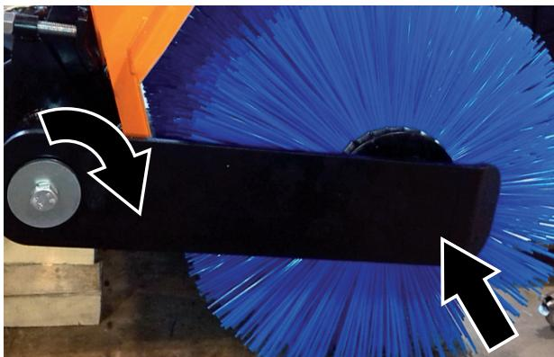
Place the brushes on the drum. Each brush has to be rotated with 90° compared to the previous one (see upper picture). If the brushes can move freely dismantle the mounted flange and add one brush and check again and add one more if needed.
