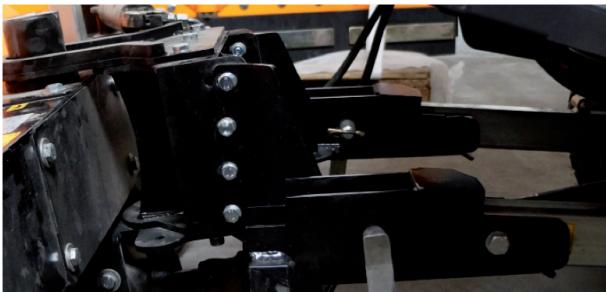
The sweep-efficiency is adjusted at the two adjustment screws on the left and right side of the support frame. Check that the sweep-efficiency is the best when the brush is tilted.
