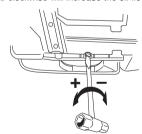
Recommended settings: Bar 13"-15": Minimum flow Bar 16"-18": Medium flow Bar -20": Maximum flow
