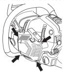
Pull out the cord approx. 30 cm (12 inches) and hook it into the notch in the rim of the pulley. Release the recoil spring by letting the pulley rotate slowly backwards.
