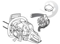
IMPORTANT! In order to maintain operation of the centrifugal cleaning system it must be regularly maintained. Clean the air intake to the starter, the fins on the flywheel, the space around the flywheel, inlet pipe and carburetor compartment.
