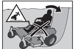
**⚠ WARNING!** Do not drive up or down hills with slopes greater than 10 degrees. Do not drive across slopes.
