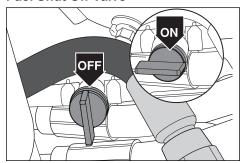
The fuel shut off valve is located at the right rear of the seat. The valve is off when the handle tab is turned perpendicular to the fuel line.
