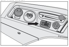
The service meter displays the total operating time with the blade activated.
