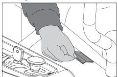
The seat can be adjusted lengthways. When making adjustments, the lever below the right side of the seat is pulled up, after which the seat can be moved backward or forward.
