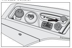
The throttle control regulates the engine speed and thereby the rate of rotation of the blades, assuming the blade switch is pulled out.
