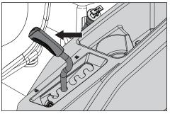
To set the deck cutting height, pull the cutting height lever inwards and move it to the desired height notch.
