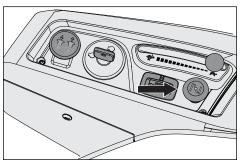
The choke control is used for cold starts to provide the engine with a richer fuel mixture. For cold starts the control should be pulled up.
