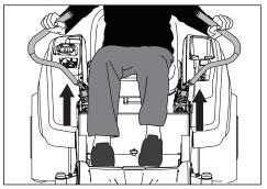
NOTE: If the steering / park brake controls are not holding in the full outboard position, the tension can be adjusted by tightening the nut on the backside of the pivot. (See Park Brake in this section).
