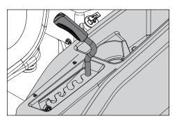
Disengage the mower blades by pressing the blade switch downwards.
