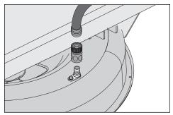
Restart the mower and engage the blades to use the spinning action to wash away debris. Make sure the hose is away from the mower blades.
