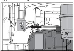
Transaxle bypass linkages must be engaged when pushing or pulling the mower. The release levers are located on each side of the rear of the unit below the rear engine guard. See *Moving Machine By Hand* in the *Operation* section.
