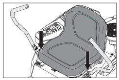
The park brake is integrated with the steering control levers. Move **both** levers out from the neutral position to engage the park brake.
