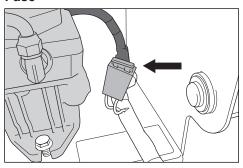
The 20 amp primary fuse is located on the left hand side of the machine. It is accessed by tilting the seat forward. The fuse is a flat pin type used in automobiles.
