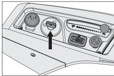
The ignition switch is placed on the control panel and is used to start and stop the engine.
