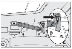
4. Turn any blade to align with the deck front-to-rear. If the front blade tip does not measure 3.175 mm to 12.7 mm higher in the rear—with a 5/8"or adjustable wrench, turn the nuts on the front suspension linkage. Clockwise raises the front of the mower, counter clockwise will lower the front. Adjust nuts until rear of mower deck is positioned level to 3.175 mm higher in the rear than the side-to-side measurement.
