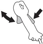
See instructions under the heading Start. Start the machine and apply full throttle. Release the throttle and check that the cutting attachment stops and remains at a standstill. If the cutting attachment rotates with the throttle in the idle position then the carburettor idle setting must
