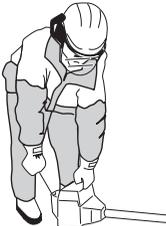
Once the engine starts operate throttle gradually to increase engine speed. Make sure the engine runs smoothly.
