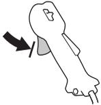
Press the throttle lockout and make sure it returns to its original position when you release it.
