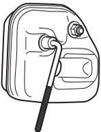
If the muffler on your machine is fitted with a spark arrestor screen this must be cleaned regularly. A blocked screen will cause the engine to overheat and may lead to serious damage.
