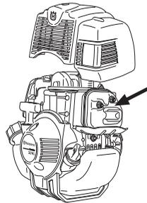
The muffler on your machine is equipped with a spark arrester screen, this should be cleaned regularly. A blocked screen will cause the engine to overheat and may lead to serious damage.
