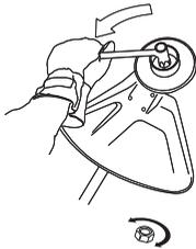
The nylon lining inside the locking nut must not be so worn that you can turn it by hand. The lining should offer a resistance of at least 1.5 Nm. The nut should be replaced after it has been put on approx. 10 times.
