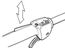
Check that the throttle trigger and throttle lockout move freely and that the return springs work properly.
