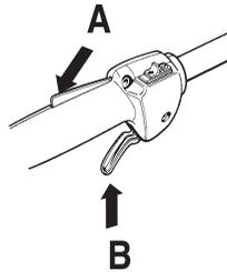
Make sure that the throttle trigger is locked at idle setting when the throttle trigger lockout is released.
