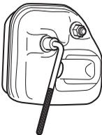
If the muffler on your machine is fitted with a spark arrestor mesh this must be cleaned regularly. A blocked mesh will cause the engine to overheat and may lead to serious damage.
