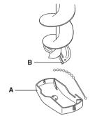
Regularly check that the transport guard is not damaged. Replace the transport guard if it is damaged.
