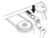
6 Lift off the drive belt and hang on the load-relieving hook.
