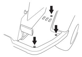
2 Loosen the locking nuts (1).
