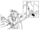
2 Replace the cutting height stay and the belt. Tension the belt with the belt adjuster.
