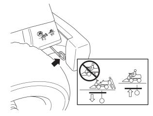
• Control drawn out, drive system disengaged. Control depressed, drive system engaged.
