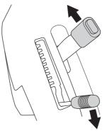
2 Release the clip on the front hood and lift off the fender.
