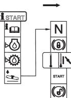
Check the engine's oil level
