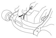
3 Loosen on the cutting height stay and place in the holder.
