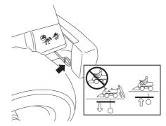
• Pull out the control to disengage the drive system. Push in the control to engage to the drive system.
