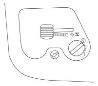
3 When the Rider is at a standstill, press down the parking brake and push in the locking button.
