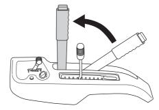
2 Move the throttle to the idle position. Turn the ignition key to the "STOP".
