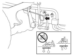
• Control drawn out, drive system disengaged.
