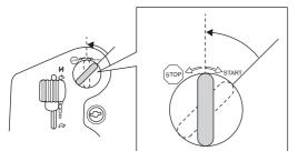
7 Move the throttle backwards gradually once the engine has started. Let the engine run at moderate speed or half throttle for 3-5 minutes before subjecting it to heavy load.
