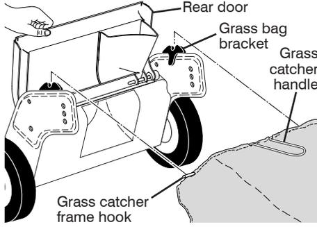
**NOTE:** Rear door will remain open until operator presence control bar is held down to the handle.
