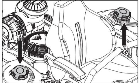
Read the safety instructions before refueling. The capacity for each tank is 22.7 litres (6 gallons).
