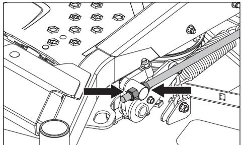
6. Be sure to check the previously measured distances to ensure that the mower deck is properly adjusted. The outer blade tip height must be equal when side-to-side. The rear blade tips must be 3.2 mm to 9.5 mm (1/8" to 3/8") higher than the front blade tip measurements when front-to-rear.
