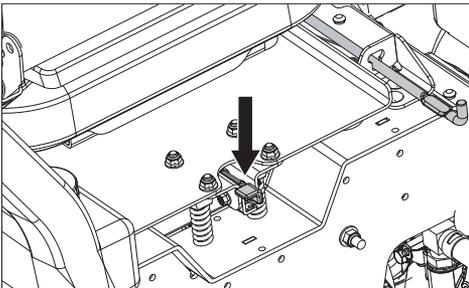
The seat can be rotated forward to access the mower battery and hydro gears. Pull up on the latch lever to release the seat. Raise the seat until the rod engages.
