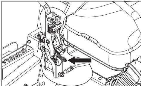
3. To change the park brake tension, tighten the pivot bolt until the desired braking is correct.
