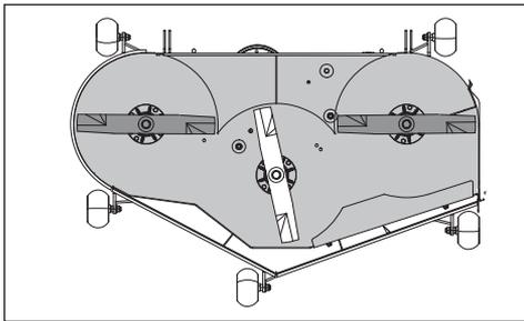
2. Measure and record the distance from ground to the bottom of the outer blade tip closest to the outside edge of the deck. Repeat this procedure for the other side. If the measurements are not the equal, adjustment is required.
