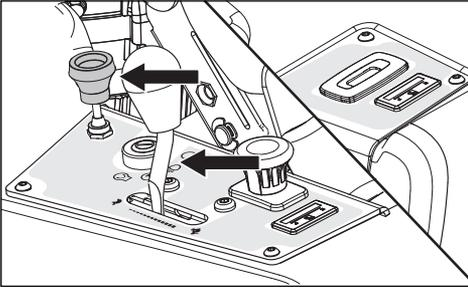
6. Set the fuel tank valve to the desired tank.
