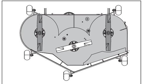
5. To set the front-to-rear deck height, adjust the locknuts on the threaded adjustment rods. Raise or lower the deck until the rear blade tips are positioned 3.2 mm to 9.5 mm (1/8" to 3/8") **higher** than the front blade tips.
