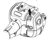
Remove the air filter cover and take out the filter. Wash it clean in warm, soapy water. Clean also the inside of the filter cover by using air or a brush. Ensure that the filter is dry before refitting it.
