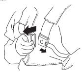
Check that the harness straps are correctly positioned. Once the harness and machine have been adjusted, check that the harness guick release works correctly.
