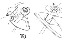
The nylon lining inside the locking nut must not be so worn that you can turn it by hand. The lining should offer a resistance of at least 1.5 Nm. The nut should be replaced after it has been put on approx. 10 times.
