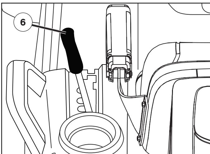
**(GB) 6. Quick lifting/lowering of the cutting unit**
