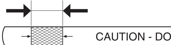
GB The oil level should lie between the two markings on the oil stick. If necessary, add oil until top of the crosshatched mark on dipstick is reached. For approximate capacity and oil type see "PRODUCT SPECIFICATIONS" section of this manual. Do not overfill.
