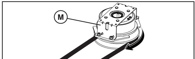
**IMPORTANT: Check belt for proper routing in all mower pulley grooves.**
