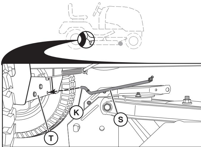
**NOTE:** Depending on model, bracket (T) may be different than shown but hole for anti-sway bar will be in same position/location.
