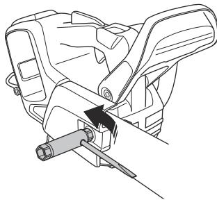
2. Lift the front of the guide bar and turn the chain tensioning screw. Use a wrench.
