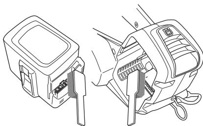
3. Make sure that the battery is not damaged and there are no other defects, such as cracks.
