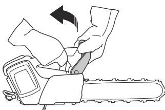
A kickback can be very sudden and intense. Most kickbacks are small and do not always engage the chain brake. If a kickback occur when you use the product, hold tight around the handles and do not let go.
