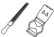
1. Use a flat file and a depth gauge tool to adjust the depth gauge setting. Only use Husqvarna depth gauge tool to receive the correct depth gauge setting and bevel for the depth gauge.
