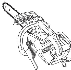
1. Clean the cooling system with a brush weekly or more frequently if necessary.
