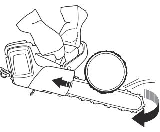
**WARNING:** Be careful when you cut on the push stroke. If the saw chain gets trapped in the trunk, the product can be pushed at you. You must prevent this force or there is a risk that the kickback zone of the guide bar touches the tree. This will lead to a kickback.
