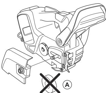
3. Put the guide bar on top of the bar bolt. Steer the guide bar to its most rear position. Lift the saw chain above the drive sprocket and engage it in the groove on the guide bar. Start on the top edge of the guide bar.
