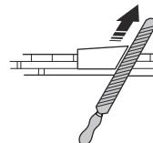
4. Remove filing material on all teeth on one side first.
