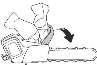
In the felling position you can not engage the chain brake manually. The chain brake can in this position only be engaged by the inertia release mechanism.
