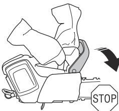
How the chain brake is engaged depends on the force of the kickback. It also depends on the position of the product when the kickback zone hits an object. If you get a intense kickback while the kickback zone is farthest away from you the chain brake engages by the inertia release. If the kickback is small or the kickback zone is nearer you the chain brake engages manually by your left hand.
