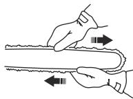
6. Do a check of the chain tension frequently until the saw chain is run-in.
