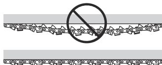
3. Move the file from the inner side of the cutting teeth and out. Decrease the pressure on the pull stroke.
