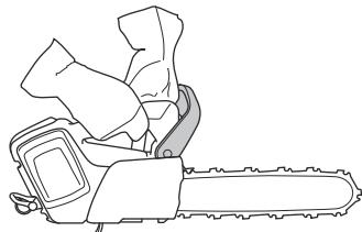
3. Apply full power and tilt your left wrist forward to engage the chain brake.
