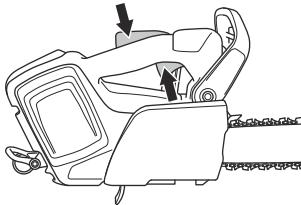
2. Press down the power trigger lockout and make sure that it goes back to its initial position when you release it.
