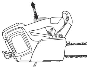
3. Make sure that the power trigger is locked at the idle position when the power trigger lockout is released.
