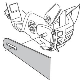
6. Make sure that the drive links of the saw chain fit correctly on the drive sprocket.
