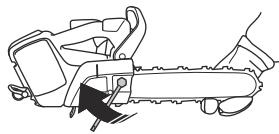
5. Make sure you can pull the saw chain around freely by hand and that it does not hang from the bottom of the guide bar.
