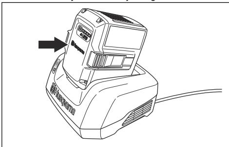
3. Make sure that the green charging light on the battery charger comes on. That means that the battery is connected correctly to the battery charger.
