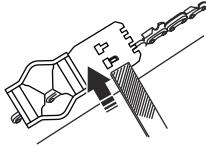
**Note:** The depth gauge setting is correct when you do not feel resistance as you move the file along the depth gauge tool.
