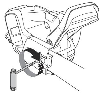
4. Tighten the bar nut(s) using the wrench and lift the front of the guide bar at the same time.
