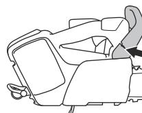
2. Make sure that the front hand guard moves freely and that it is attached safely to the product.
