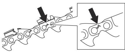
2. Examine if the saw chain is rigid. Replace if necessary.
