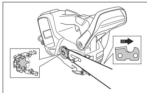
4. Make sure that the edges of the cutting links are turned forward on the top edge of the guide bar.
