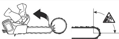
Kickback always occurs in the cutting plane of the guide bar. Usually, the product, guide bar and saw chain are thrown against the operator but can also move in a different direction. It is how you use the product when the kickback occurs that causes the direction of movement.
