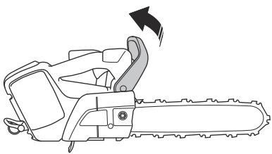
2. Remove the bar nut, the drive sprocket cover and the transportation ring (A).
