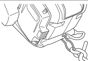
**Note:** If the operator loses control of the product, the strap will prevent the product from falling to the ground. Attach the belt eyelet to the hook on
