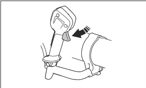
2. Push the Cruise control button to set the selected airflow. The LED comes on.
