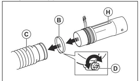
5. Make sure to put the clamp screw (D) as the illustration shows. Tighten the screw.
