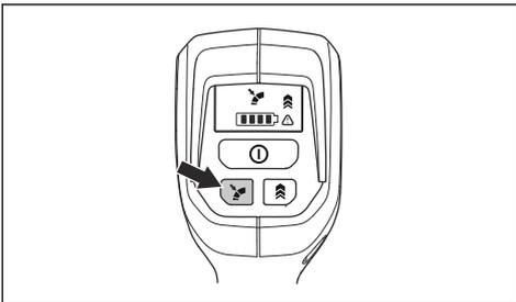
3. Continue to operate with the selected airflow without the power trigger pushed.
